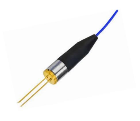
The FCML series diode lasers deliver up to 50mW of power through a 50/125μm fiber. They feature built-in optical isolator, low capacitance and low dark current, high stability, low threshold current, low operating current, integrated high isolation, and low insertion loss.
